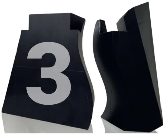
Complex geometries in the manufacturing of samarium-cobalt magnets – setting new standards in magnet technology
