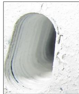
Fig. 4 Photograph of a slot in a test lamination stack, after the application of the proprietary ceramic coating.
